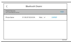
10. Once paired, the Control Panel displays the connected device, its MAC, Partition assignment and its connection status. There is the option to "UNPAIR" or toggle the disarm feature on and off for the user's device.
