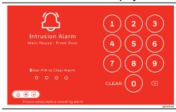
Intrusion alarms are accompanied by a solid tone from the Control Panel, Touchscreens, Keypads, and Sirens. It displays the partition name (if partitions are enabled) and the first sensor that activated the alarm along with a Keypad to enter a valid code to disarm and acknowledge the alarm. Once a code is entered, all alarm sounds are silenced. To view any additional sensors that went into alarm, see the system's Activity Log.
