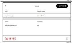
6A. "Test Wi-Fi" provides information such as the name of the network it is connected too, Signal Strength in dBm, speed, and internet connection.
