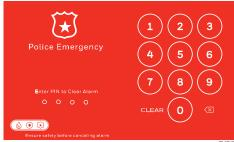
4. Enter a valid 4-digit code in the displayed keypad to acknowledge the alarm and silence the alarm sounds.
