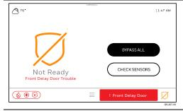
To acknowledge any Alert, simply touch the red box at the bottom of the screen and any existing beeping stops.
