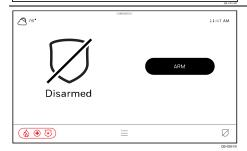
When all sensors are closed and there is no activity, no faults are displayed, and the system reflects a simple "Disarmed" state. This means the system is "Ready to
