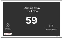
The system reflects the arming mode and the time remaining in the Exit Delay countdown.
