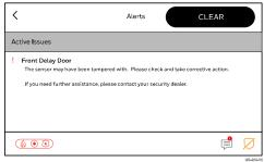
2. If the condition still exists after acknowledging it, it is listed as an "Active Issue" and remains on the display as a bubble at the bottom-right indicating how many Alerts are still active.
