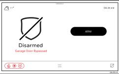
Once all faulted sensors are bypassed, the option to arm the system is displayed. Select to choose your arming mode. See "Choosing your Arming Mode" Later in this section.
