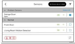
A list of all sensors is displayed, which also indicates any sensors that are faulted. The "Normal" sensors are sensors that are not faulted. Select to filter the view of the sensors by Status, Name or Device Type. This example displays by "Status". The same list of sensors can be accessed by selecting from the Home screen, then, select "Sensors" ((•)).
